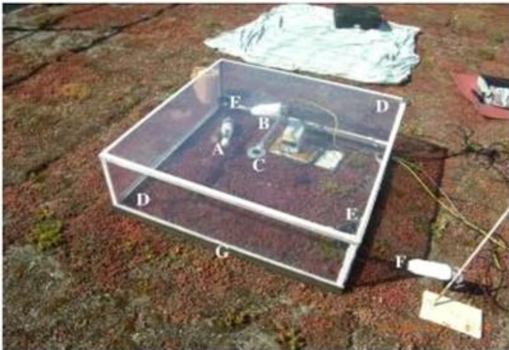
Figure S.4: Evapotranspiration chamber developed at CEREMA. The letters are defined as follows: A for Absolute humidity measure; B and F for respectively indoor and outdoor temperature sensors; C for net radiation sensor; D: PMMA enclosure and, E for the fan (Sabre et al., 2015).
